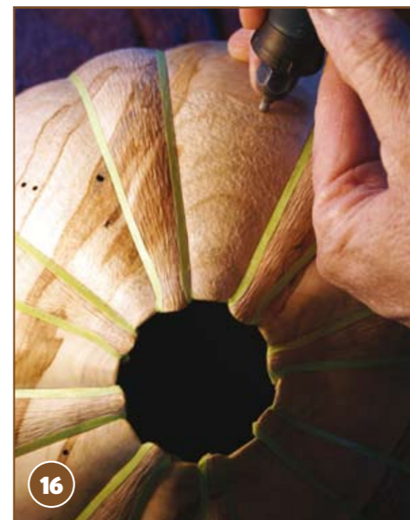
16 A small polished point is used in the reciprocating tool to “stipple” or “hammer” the smooth, finished surface. It's not a terribly complicated technique, but requires some practise to learn to vary the touch in different grain areas so the look is the same. End-grain hammers differently than side-grain and so forth
