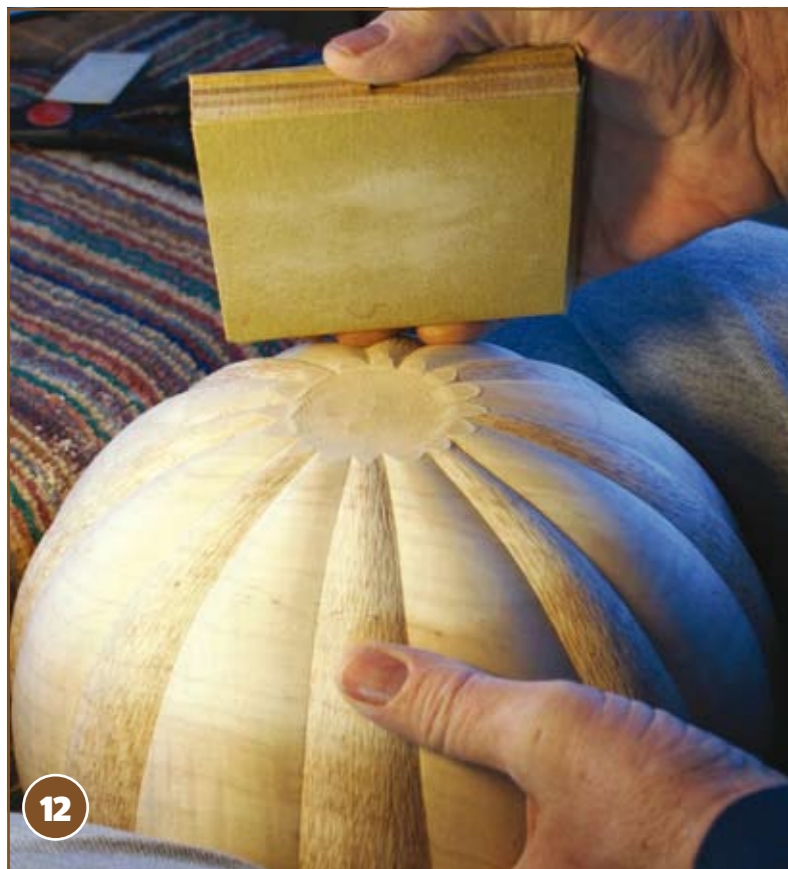
12 Next, I flatten the bottom with a sanding block and carve the bottom with a small gouge, until it is slightly concave in shape.
