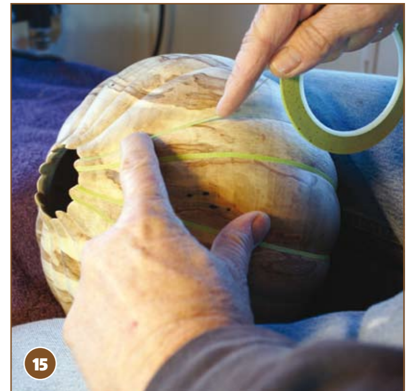
15 The textured narrow bands are taped off with fine-line masking tape, which prevents damage from “stippling” or “hammering” in the next step
